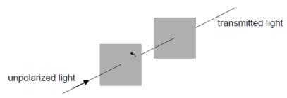
The first polarizer is now rotated about the direction of the incident beam by an angle smaller than 90°. Which gives the changes, if any, in the intensity and polarization of the transmitted light?
