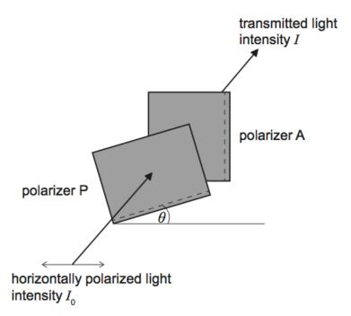
The angle  $\theta$  is varied from 0 to 90 degrees. Which of the following represents the variation with  $\theta$  of the intensity / of the light transmitted through A?
