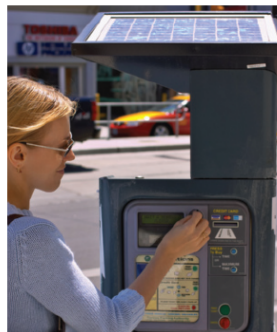
Figure 11 A parking meter uses electrical energy produced by a solar cell.
